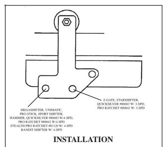
**Note:** Be careful. Select the correct hole for your shifter. Wrong hole will destroy the cable, shifter and/or transmission in **one** shift! (GM trans. only)
