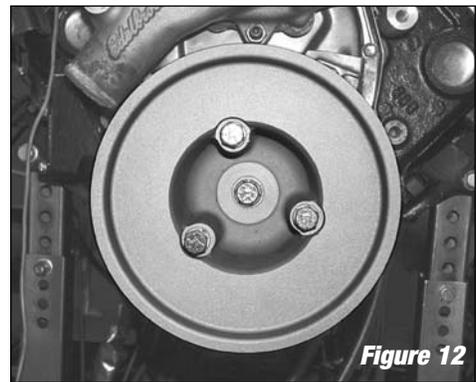
**10. Install the supercharger snout support/idler pulley bracket:**
