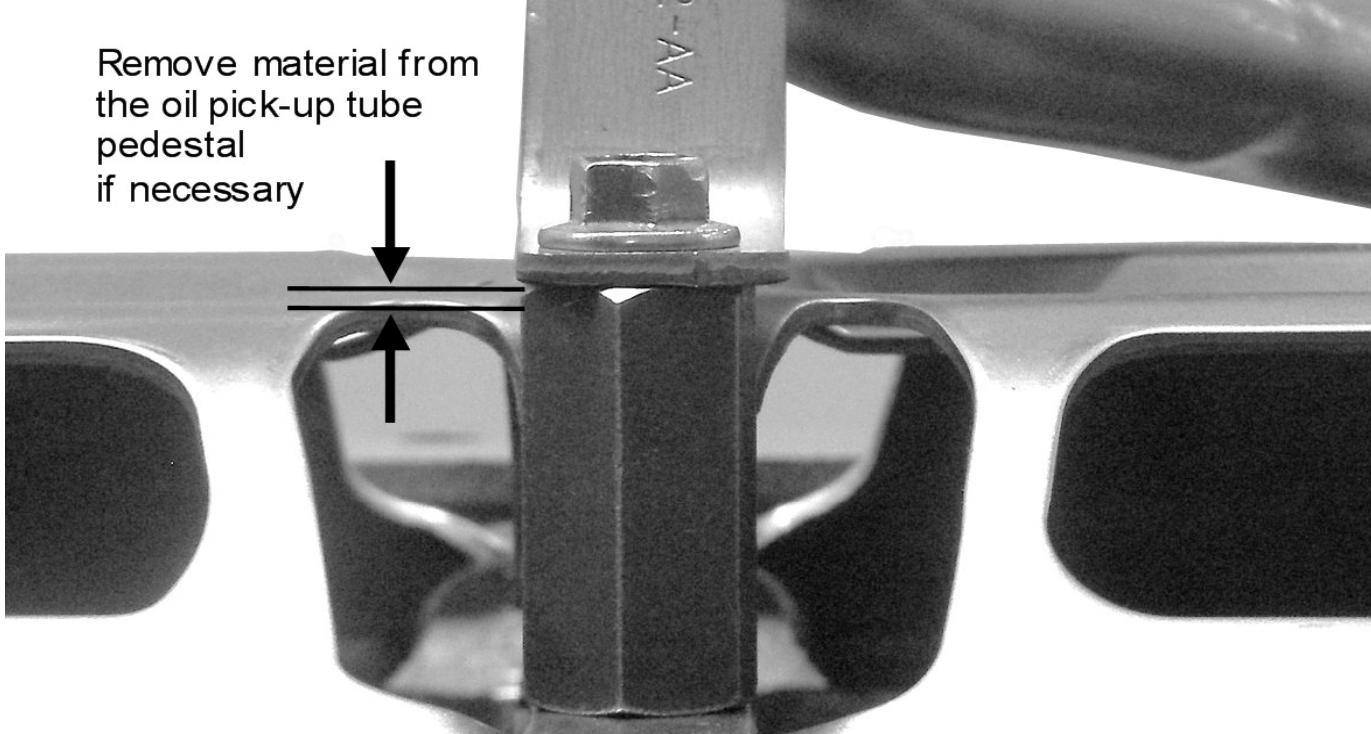
1. When using the OEM oil pan and pick-up tube it will be necessary to shorten the oil pick-up pedestal by .070 in. to set the oil pick-up tube back at the stock height.
