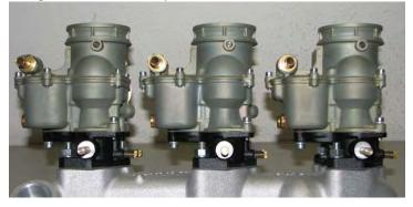
2. Rotate each arm so that it will point back at roughly a 45° angle. Use a straight edge to ensure that the linkages are installed at the same depth on the throttle shafts and that the throttle arms remain parallel throughout the full range of pedal travel. It may be necessary to loosen the carb nuts and adjust the carbs' position in order to achieve the correct alignment.
