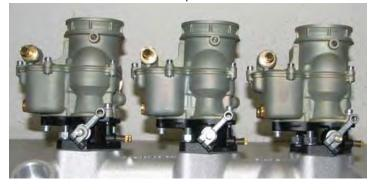
4. Install the swivel studs in each of the linkage arms so that the set screws point away from the carburetors. Slide a washer over the back of the swivel studs then secure each of them with a cotter pin.
