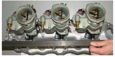
3. Once the correct angle and depth have been achieved, tighten the set screws to secure the arms to the shafts. Twist each linkage to make sure that the arms will not slip on the shafts.
