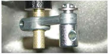
5. Install the long linkage rod through all of the swivel studs and tighten the philips head set screw on each of the swivel studs. Verify that the linkage is able to operate the carburetors throughout their full range of movement.
