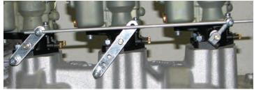
8. Install the capped rod, with the capped end forward, through the front and center carburetor swivel studs being sure to install the floating stop between. Leave roughly 1.5" between the rod cap and the front carburetor's swivel stud then tighten the swivel stud set screw on the center carburetor's throttle arm. Do not tighten the set screw on the floating stop at this time. *NOTE: Capped rod may require trimming to clear the manifold.*
