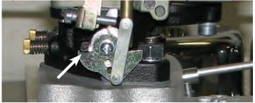
10. If the front and rear carburetor's throttle blades fail to reach wide open, loosen the swivel stud set screw on the center carburetor's throttle arm and decrease the gap between the rod cap and the swivel stud on the front carburetor. Retighten the swivel stud set screw on the center carburetor's throttle arm and repeat the test.
