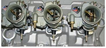
2. Install the three throttle arms as close to the carb body as you can without causing interference. The largest arm goes on the center carb with the single hole on top, while the arm with three holes goes on the front carb and the arm with two holes goes on the rear carb.
