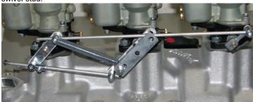
17. Vehicles using a passenger side linkage may attach the back side of the spring to the lower hole on the center carburetor's throttle arm that is not occupied by the threaded swivel stud.
