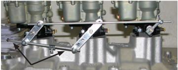
9. Twist the throttle arm on the center carburetor to wide open then inspect the other side to see that the pump cam is against the stop.
