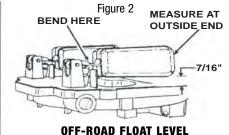
With bowl cover inverted, bowl cover gasket in place, and weight of float seating needle, there should be 7/16" between top of each float and bowl cover gasket (at outer end). The sides of floats should be parallel to the outer edge of the bowl cover. To adjust, bend float lever.
