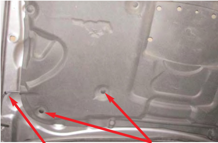
Detach hose retaining clip, then remove these two pins.
