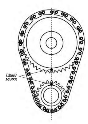
Figure 2- Timing Chain Sprocket Alignment
