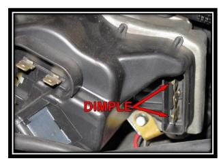
**BLACK:** 18 gauge wire, printed [WIPER MOTOR] #979 LOW/PARK, this is a signal to the low-speed tab on the wiper motor.
