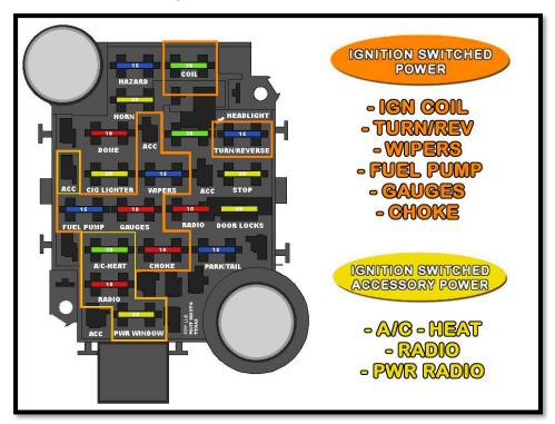
The drawing above shows all the switched ignition fuses. These fuses are powered by wires coming from the ignition switch (wires **#931**, **#932**, and **#933**) and receive power depending on what position the ignition switch is in. None of these fuses should have power when the ignition is in the *OFF* position. The <u>Ignition Switch Section</u> beginning on page 81 of this manual will go into further detail about power supplied to these fuses.
