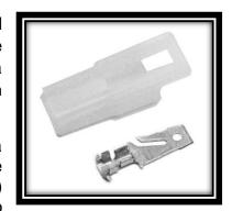
**Factory Switch:** The factory wire for the switch has a single terminal installed into the side of the switch. This wire can be difficult to remove, and, chances are, you will break the switch trying to remove it. Painless recommends cutting the wire going to the switch and installing a terminal and connector, as seen in the photo below. This allows the connector shown above to be installed on the Painless harness and plug right in.
