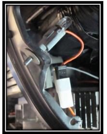
• With the factory switch now modified, install it into the dash and connect it to the **ORANGE #971** wire on the Painless harness.
