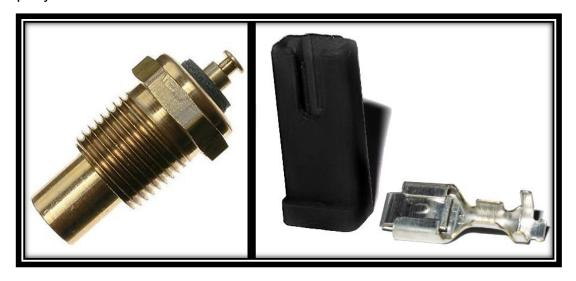
Two-wire temperature sensors on fuel injected engines are for engine computer input, not for gauge signal. Also, if connecting to an engine in a vehicle that has electric cooling fans, make certain you know the difference between the coolant temp sensor and the electric fan thermostatic switch. Both of these sensors can look identical.
