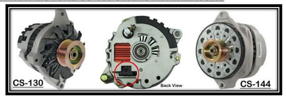
The CS-130, CS-121, and CS-144 alternators closely resemble the SI series alternators. They have an external fan behind the pulley and, generally, a plastic casing on the side and back. These alternators have a 4-pin, sealed connector, shown in the photo below and circled in the image above. The regulator will be marked P, L, S, F. This type of alternator was used on GM TPI and LT1 fuel injected engines among other late 1980's to mid-1990's GM vehicles.
