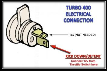
of the throttle switch and cut to length. Use terminals from the parts kit to connect the wire.
