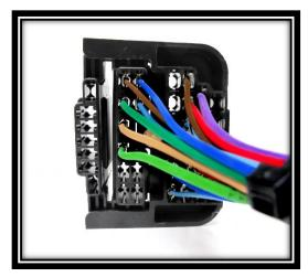
In order to utilize these switched power sources, you must add wires to the engine harness bulkhead. Terminals have been provided in the parts kit for these connections (see page 22). These terminals will accept 18-14 gauge wire, using a ½" strip length, and will need to be installed with roll-over style crimpers as shown on page 4.
