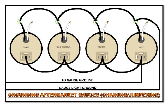
Gauge light power is supported by the GREY #930 wire. This wire connects to one of the leads for the gauge light or to the gauge light tab found on gauges with LED backlighting. To make these connections you can splice from this GREY #930 wire to all the gauges or chain/jumper it all together.
