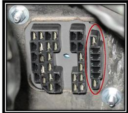
The ignition switched power on these (2) pins comes directly from the ignition switch. These pins are both **UNFUSED** and must have an inline fuse (**not supplied**), no larger than 10 amps, installed before being routed to a component needing power.
