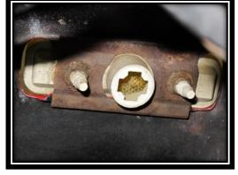
route the LT. BLUE #926 wire to the BLACK wire of the socket and cut the #926 to length, save the cut off piece of #926.
