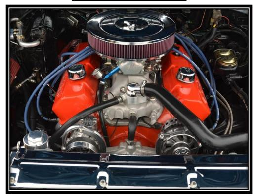
The <u>Engine Section</u> consists of five wires. They connect to the tachometer, oil pressure and coolant temperature sending units for gauges or lights, the coil or ignition system, and an electric choke on a carburetor. Locations of all of these components will vary from vehicle to vehicle, so no specific routing instructions can be given.
