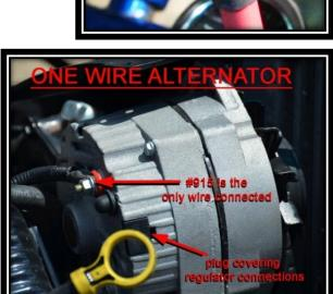
RED: 14 gauge wire, printed [ALTERNATOR] #995 REGULATOR POWER (BATTERY), this is the sense wire, it provides a battery power source, or voltage sense, that all voltage regulators require. This wire has power at all times and comes from the large battery supply splice in the harness. This wire will not be needed if you have a one wire alternator or a GM CS series alternator. See the various alternator illustrations on pages 54, 56, 58, & 59 and the Charge/Battery Power Schematic on page 63.
