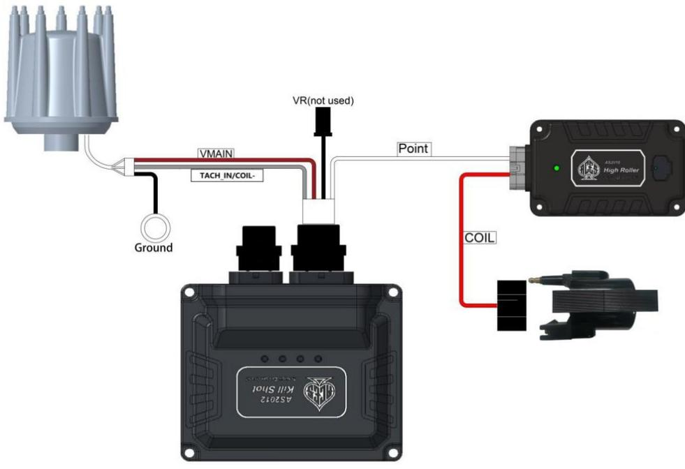
The loose wire “Point” provides an ignition signal from the KILLSHOT™ ECU to another module like the ACES HIGH ROLLER™ CDI box.
