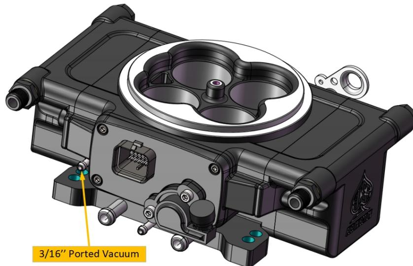
3) Reconnect all vacuum hoses, being sure to connect any ported vacuum systems to the correct 3/16" port as shown above. Leave any unused ports capped with the provided rubber caps.
