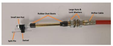
**9.** Thread the swivel & pin onto the cable to about the middle of the threaded section, then reinstall, but do not tighten the jam nut at this stage. Before proceeding, verify that forward gear selector pin and C-Clips are installed in the correct position that is required for you application.
