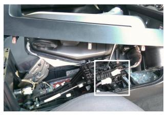
On the passenger side of the console, find and disconnect the electrical connector. Then lift the shifter boot off the shifter stick. NOTE: Leave the emergency brake connected to its boot.
