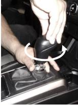
Separate the trim ring from the shifter handle by pushing down on both sides of the shifter boot.
