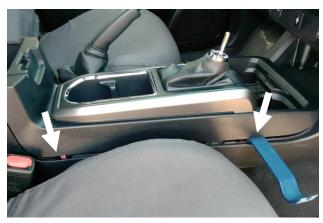
Open the center console storage compartment lid and fully engage the parking brake. Then use a plastic trim tool to carefully separate the center console from its base.
