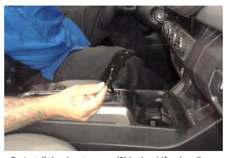
Install the six set screws (5) in the shifter handle – three screws on each side. Align the handle as desired, then tighten the set screws.
