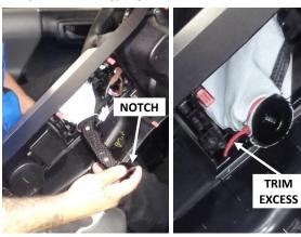
5. Work the shifter handle (item 1) up through the boot until the its opening surrounds the notch at the base of the handle. Use the supplied cable tie to secure the boot to the handle. Trim the cable tie.
