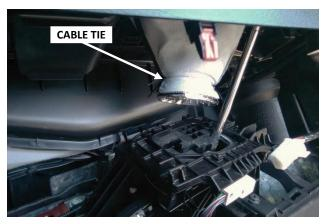
Push the shifter boot to underneath the console.
