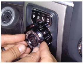
7. Set knob insert onto shifter knob and push until it is fully seated.
