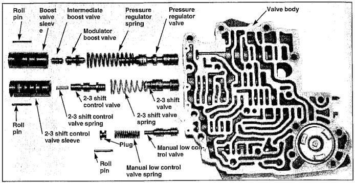
sleeve assembly as removed. Align sleeve and install retaining roll pin.
