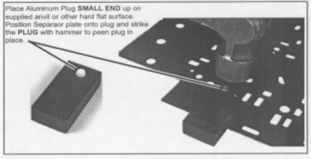
Figure 6. Separator Plate, Aluminum Plug Installation
