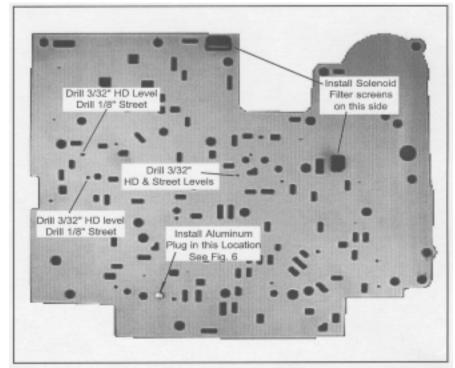
Figure 5. Separator Plate
