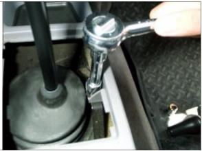
STEP 23. Install center console bolt in cup holder. <u>Tools:</u> Drive, extension, 10mm socket.
