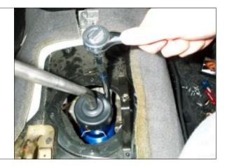
STEP 19. Reinstall rubber protective boot.
