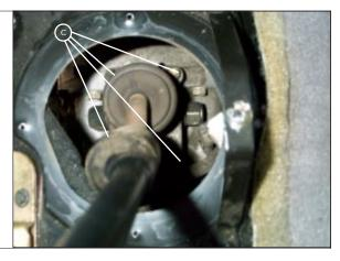
STEP 14. Pry pivot cup from stock shifter. <u>Tool:</u> Screwdriver (flat)
