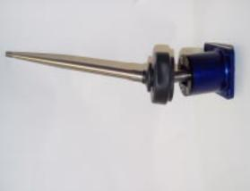
STEP 17. Either reuse stock gasket or apply RTV silicone sealant to shifter base.
