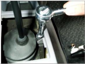
STEP 6. Remove center console bolt in cup holder. <u>Tools:</u> Drive, extension, 10mm socket
