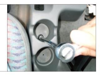
STEP 24. Install center console bolts from storage console (a)
