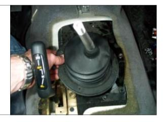
STEP 20. Reinstall rubber protective boot bolts. <u>Tools:</u> Drive, extension, 7mm socket.
