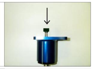
STEP 16. Install Rubber boot and ring on shifter base.
