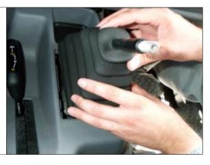
STEP 5. Remove center console bolt near shifter. <u>Tools:</u> Drive, extension, 10mm socket
