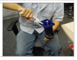
STEP 18. Install B&M Short Throw Shifter. <u>Tools:</u> Drive, extension, 12mm deep socket.
