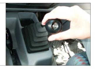
STEP 28. Install shift knob jam nut. <u>Tools:</u> Drive, extension, 15mm socket .
