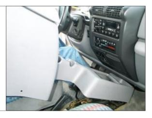
STEP 22. Install center console bolt near shifter. <u>Tools:</u> Drive, extension, 10mm socket.
