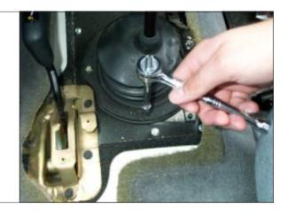
STEP 12. Remove rubber protective boot. <u>Tools:</u> Screwdriver (flat)
