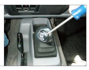
STEP 2. Remove stock shift knob jam nut. <u>Tools:</u> Drive, extension, 15mm socket
