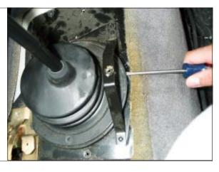
STEP 13. Remove bolts securing shifter to transmission. <u>Tools:</u> Drive, extension, 12mm deep socket
