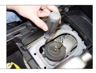
STEP 10. Remove bolts (4) and screws (3) holding down shifter.
