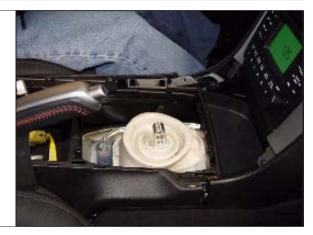
STEP 16. Install top stick (L)using (2) 5/16-18 bolts and thread adhesive.
