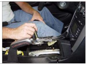
STEP 12. Remove bolts (2) holding down GTO trans base. TOOLS: 6mm Hex, Extension & Drive
