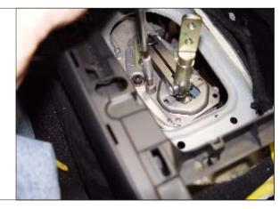
STEP 11. Pull out entire stock shifter assembly, including o-ring.
