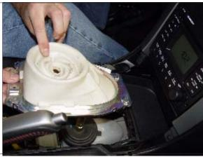
STEP 9. Remove torx screws (4) holding down shift cover and remove.
