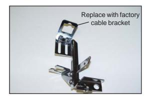
Step 2: Mount the TPS to firewall or inner fender in an area where the cable will not be in a bind.
