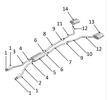
**STEP 1:** (Carefully read all instructions before installation) Disconnect the vehicle's battery before removal of the OEM exhaust system. This will prevent electrical accidents and will reset the computer if it applies to the vehicle. Remove existing exhaust system from the vehicle. Only remove parts that will be replaced. Clean existing flange with a wire brush to ensure proper sealing.
