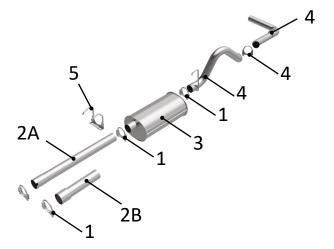
2A: 131" Wheelbase (123.9" Wheelbase Cut to fit)
