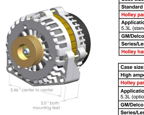
Case size: SMALL (130 mm) Standard amperage: 105 AMPs Holley part # 197-300 **Application:** '04 Chevy Silverado 5.3L (standard 105 amp choice) GM/Delco # 10480326 Series/Lester # AD230/8247 Holley harness pigtail # 197-400 Case size: LARGE (144 mm) High amperage: 130-145 AMPs Holley part # 197-301 **Application:** '04 Chevy Silverado 5.3L (optional 130/145 amp choice) GM/Delco # 15754097 Series/Lester # AD244/8292 Holley harness pigtail # 197-400
