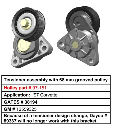
The above is the only style of tensioner that will work with the Holley bracket kits. The recommended version is common on 1997 - 2004 Corvettes. GM tensioner # 12569301 found on 2005 and up Corvettes may also be used if salvaged from the donor accessory drive, but confirm the tensioner pulley properly aligns with the belt after installation.
