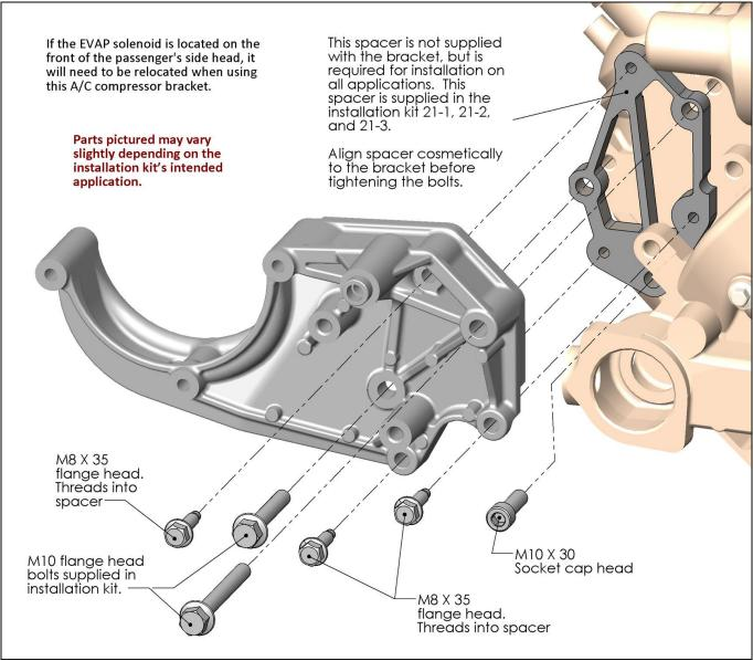
NOTE: Torque M8 bolts to 18 ft./lbs. and M10 bolts to 36 ft./lbs.
