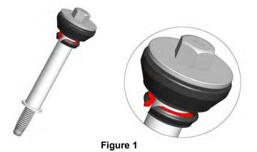
**NOTE:** Aged grommets will likely tear during the removal and reinstallation processes. The area that is affected is only for temporary retention during installation and will not hurt the sealing function of the grommet.
