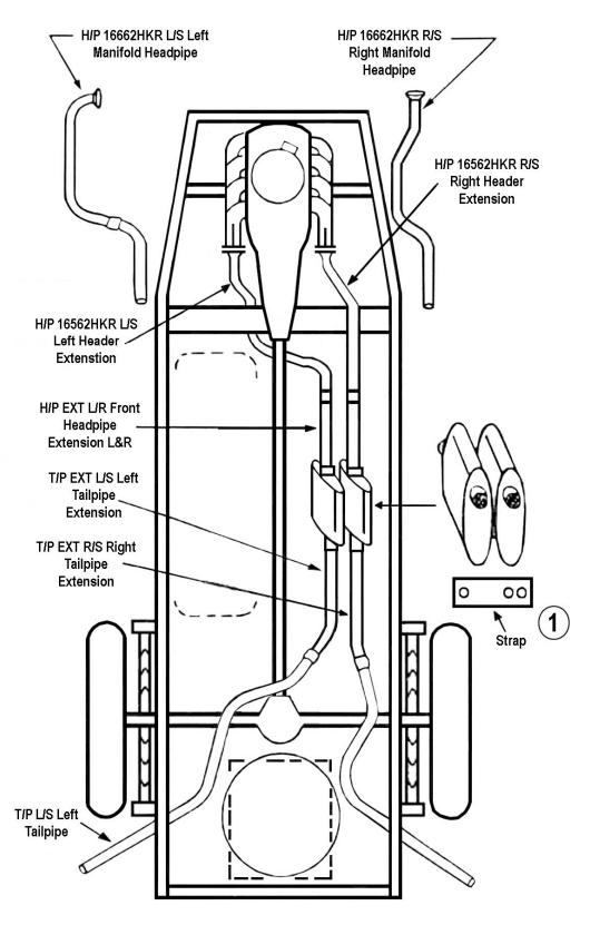
Install mufflers side by side in this position with center inlet in front. Use 3-hole straps & U-clamps for proper clearance between mufflers & pipes.
