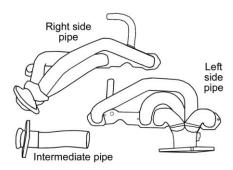
WARNING! Breaking in an engine with ceramic-coated headers WILL result in damage to the coating and will VOID all warranties. Ceramic-coated headers require several heat cycles to fully cure before they will withstand extreme heat. HOOKER recommends using a cast-iron exhaust manifold or an old header to break in new engines to avoid coating damage.
