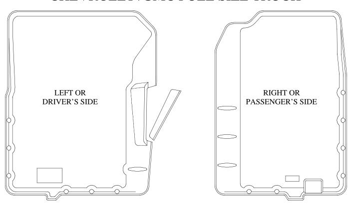
IF YOUR VEHICLE IS EQUIPPED WITH A MANUAL TRANSFER CASE SHIFTER, YOU WILL NEED TO TRIM YOUR DRIVER'S SIDE LINER BEFORE INSTALLATION (SEE DIAGRAM ABOVE). USING A UTILITY KNIFE OR SCISSORS, CAREFULLY REMOVE THE RECESSED PORTION OF THE LINER WALL. ONCE TRIMMED, YOUR LINER WILL CONTOUR THE SHIFTER HOUSING
