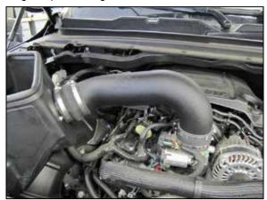
14. Install the K&N<sup>®</sup> intake tube into the hump coupler at the filter adapter and then into the coupler at the throttle body, adjust the tube for best fit and then secure with the provided hose clamps.
