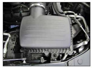
4. Pull up the factory air filter housing to dislodge it from the mounting grommets and then remove the complete intake assembly from the vehicle. NOTE: K&N Engineering, Inc., recommends that customers do not discard factory air intake.
