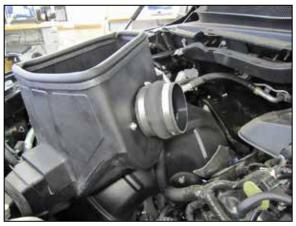
10. Install the provided hump coupler (08418) onto the filter adapter and secure with the provided hose clamp
