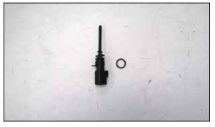
12. Remove the inlet air temperature sensor from the factory intake tube and then remove the O-ring from the sensor.
