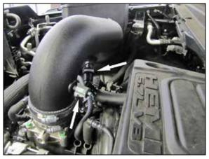
15. Reconnect the inlet air temperature electrical connection. Connect the factory crank case vent line to the quick disconnect fitting installed into the K&N<sup>®</sup> intake tube.
