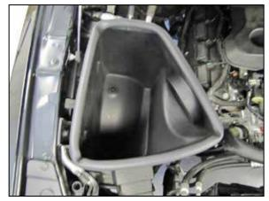
8. Install the K&N<sup>®</sup> air filter housing into the vehicle so the grommets fit onto the factory mounting posts.
