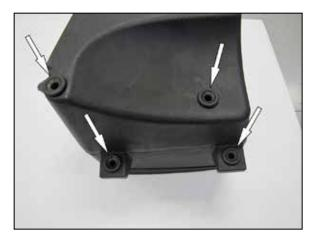
7. Remove the four mounting grommets from the factory air filter housing and install them into the K&N<sup>®</sup> housing as shown.
