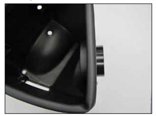
6. Install the filter adapter into the K&N<sup>®</sup> air filter housing and secure with the provided hardware.
