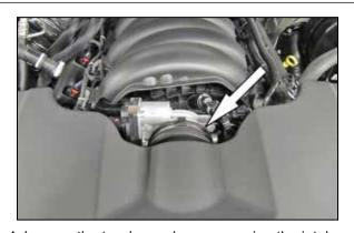
4. Loosen the two hose clamps securing the intake plenum to the factory air box and to the throttle
