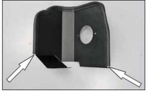
8. Install the provided edge trim onto the heat shield as shown.
