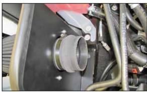
14. Install the provided coupling hose (08699) onto the filter adapter and secure with the provided hose
