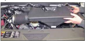
5. Remove the intake plenum from the vehicle.
