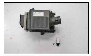
15. Remove the two screws securing the mass air sensor to the factory air box and then remove the sensor from the air box.
