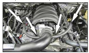
19. Install the provided crank case hoses onto the valve cover ports and then onto the fittings in the K&N® intake tube.
