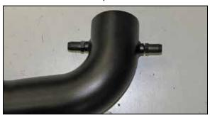
17. Install the two provided crank case vent fittings into the K&N® intake tube as shown.
