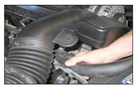
4. Unhook the radiator hose mount from the intake tube.
