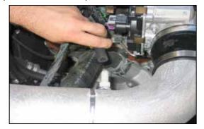
25. Install the provided crank case vent hose onto the valve cover vent port and then connect the remaining open end to the  $\frac{1}{4}$ " NPT fitting in the K&N<sup>®</sup> intake tube.
