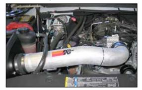
24. Install the K&N<sup>®</sup> intake tube into the silicone hose at the filter adapter and then into the silicone hose at the throttle body, then secure with the provided hose clamps.
