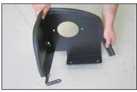
12. Install the provided edge trim onto the heat shield as shown.
