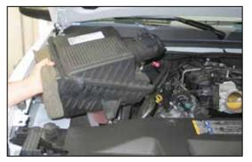
8. Pull firmly upward to release the air cleaner assembly from the mounting tray grommets. Then
