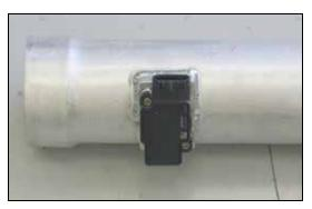
10. Install the mass air sensor into the  $K\&N^{\otimes}$  intake tube and secure with the provided hardware.
