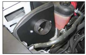
20. Install the filter adapter onto the heat shield and
