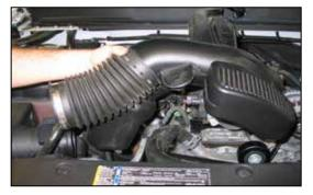
6. Loosen the hose clamp, which secure the stock intake tube, then remove the intake tube from the vehicle.
