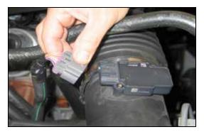
2. Disconnect the mass air electrical connection.
