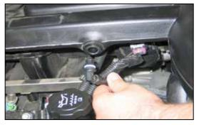
5. Unhook the crank case vent line from the intake tube plenum as shown.
