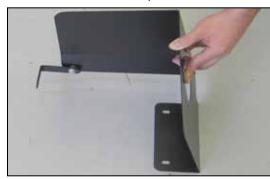
11. Install heat shield mounting bracket (010031) onto the heat shield as shown using the provided hardware.
