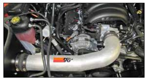
18. Install the K&N $^{\mbox{\tiny B}}$  intake tube into the hose at the
