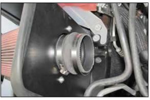
14. Install the coupling hose (08699) to the filter adapter and secure with the provided hose clamp.
