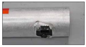
16. Install the mass air sensor into the K&N<sup>®</sup> intake tube and secure with the provided hardware.
