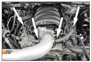
19. Connect the provided crank case vent hoses to the ports on the valve covers and then connect the open ends to the fittings installed into the K&N<sup>®</sup> intake tube and secure with the provided hose clamps.
