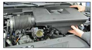
5. Remove the intake plenum from the vehicle.
