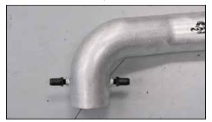
17. Install the two provided crank case vent fittings into the  $K\&N^{\circledast}$  intake tube as shown.
