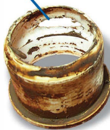
WORN, FAILED BEARING
