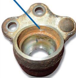
CORROSION IN HOUSING INDICATING INTRUSION
