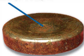
CORROSION IN HOUSING INDICATING INTRUSION
