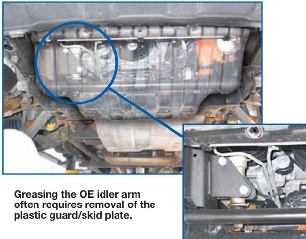
Greasing the OE idler arm often requires removal of the plastic guard/skid plate.
