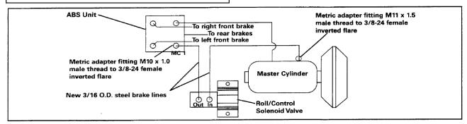
Use only SAE approved seamless steel brake lines with double flared ends that are of the correct size and length, and come preassembled with inverted flare tube fittings. DO NOT CUT brake lines. DO NOT USE copper tubing. When bending brake lines, use a tubing bender to avoid kinking or crushing. Use thread sealer on threaded fittings. A line fitting wrench is recommended to be used when tightening all brake line fittings.
