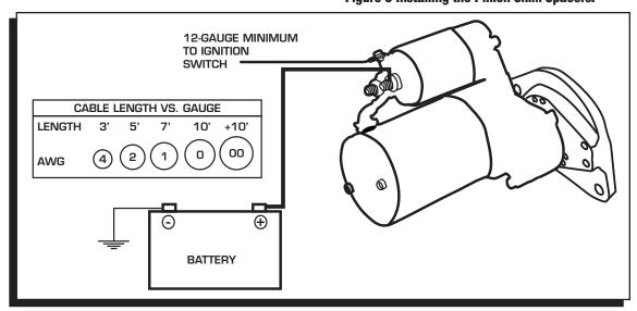
Figure 4 Wiring the DynaForce High Speed Starter.
