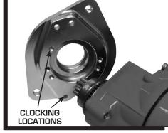
Figure 1 Clocking the Starter for Clearance.
