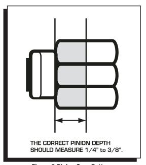
Figure 6 Pinion Gear Pattern.
