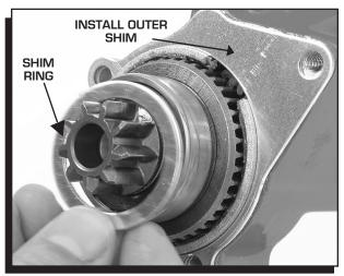
**Figure 3 Installing the Pinion Shim Spacers.**
