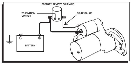
Figure 5 Wiring to Incorporate an External Solenoid.
