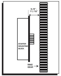
Figure 2 Checking Pinion Clearance.
