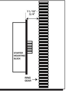
Figure 2 Checking Pinion Clearance.
