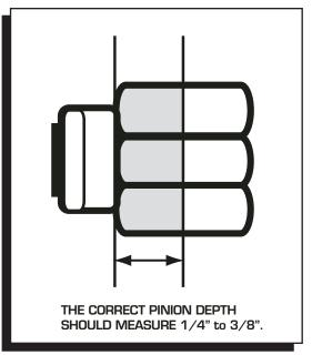
Figure 6 Pinion Gear Pattern.
