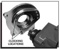
Figure 1 Clocking the Starter for Clearance.
