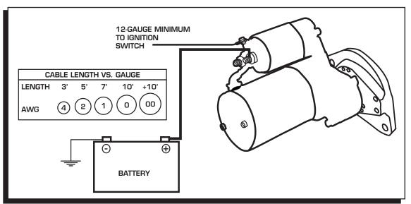
Figure 4 Wiring the Starter.
