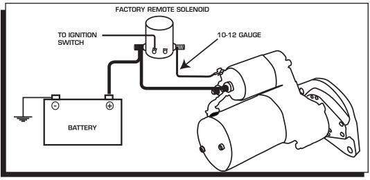
Figure 5 Wiring to Incorporate Factory Solenoid.
