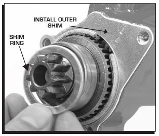
Figure 3 Installing the Pinion Shim Spacers.
