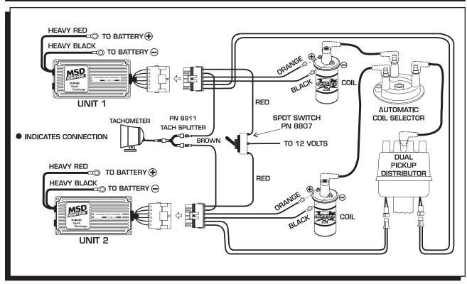
Figure 4 Two MSD 6 Series and Coils with a Dual Magnetic Pickup Distributor.
