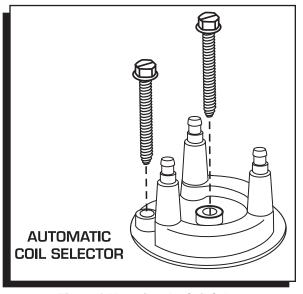
Figure 1 Mounting the Coil Selector.
