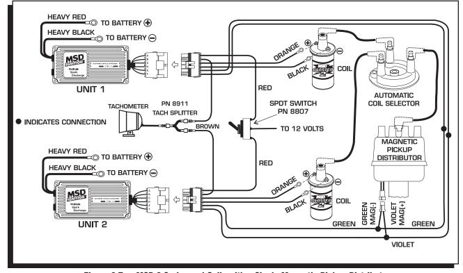
Figure 3 Two MSD 6 Series and Coils with a Single Magnetic Pickup Distributor.
