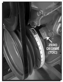
Figure 9 The Timing Tape Installed.
