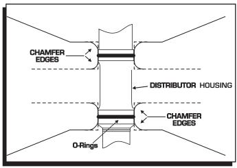
Figure 6 Modified Block for use with O-Rings.
