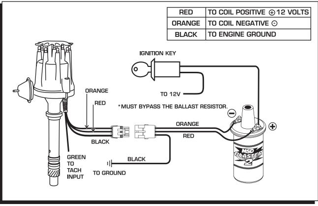
Figure 7 Wiring the Ready-to-Run Chevrolet Distributor.
