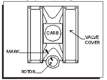
Figure 5 Marking the Rotor Location.
