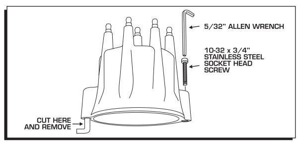
Figure 10 Optional Installation by Bolting the Cap Down.
