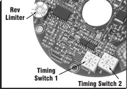
Figure 1 Rotary Dial Adjustments.
