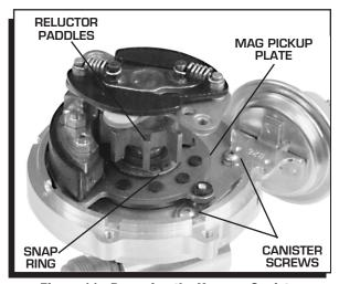
Figure 11 Removing the Vacuum Canister.
