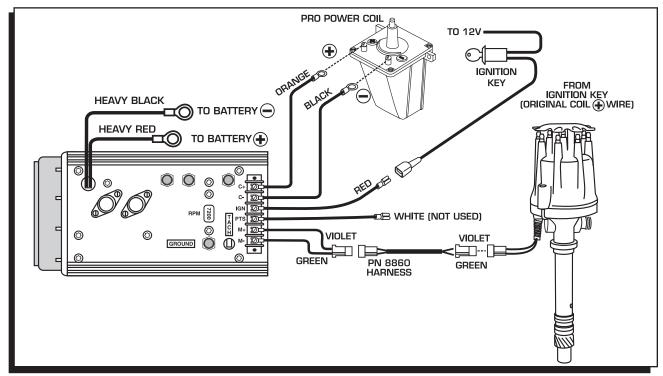
Figure 14 Wiring to an MSD 7-Series Ignition Control.
