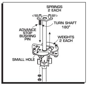
Figure 7 Locking Out the Advance.
