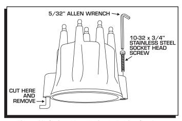
Figure 10 Optional Installation by Bolting Cap Down.
