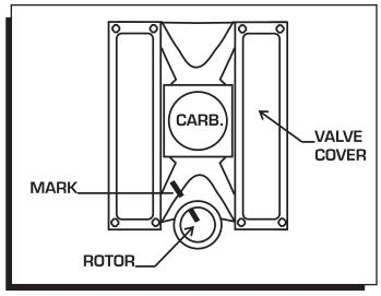
Figure 8 Marking the Rotor Location.
