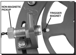
Figure 2 - MSD Flying Magnet Crank Trigger.
