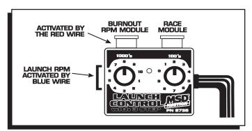
Figure 1 Module Controls and Adjustments.
