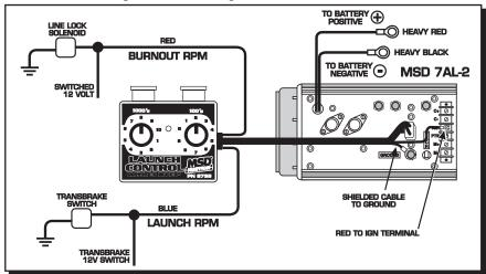
Figure 3 Wiring with an MSD 7 Series Ignition.
