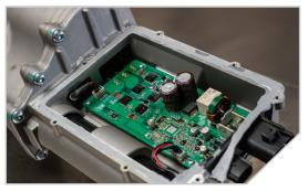
Coated electronics to prevent water intrusion and corrosion
