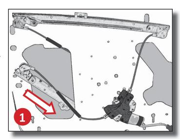
**STEP 2:** Insert the top of the right rail into the right hole. The end of the rail will slide up between the glass and the door to allow the bottom of the rail to be inserted. Mount the rails to the door loosely. Attach the glass to the regulator and adjust the rails for proper alignment.
