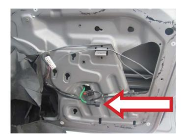
**STEP 8:** Remove the window regulator assembly through the access hole below the speaker hole.
