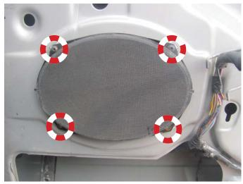
**STEP 6a:** Disconnect the door speaker connector from the door speaker.
