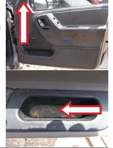
**STEP 1a:** Using a Torx bit (T-25), remove the interior door handle bezel. **NOTE:** Some vehicles used a T-15 and a T-25 Torx bit.
