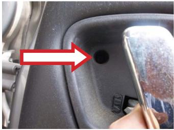
**STEP 12:** Verify that all of the interior door trim panel retainers are secure and that the window regulator is operating properly.
