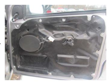
**STEP 4a:** Remove the water shield from the door.
