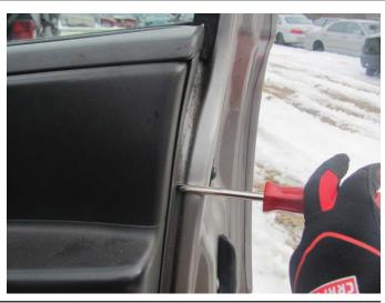
**STEP 3:** Disconnect the door latch rod retainer clips from the door latch rod.
