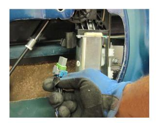
**STEP 8:** Remove the six 10mm window regulator mounting bolts that secure the window regulator to the door frame.
