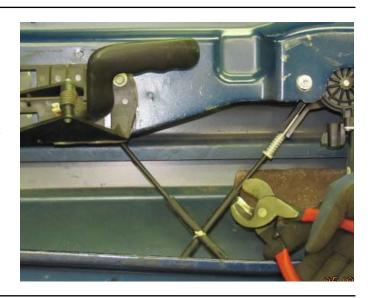
**STEP 5:** Loosen the 10mm window guide bolts enough so that the window can be separated easily from the clamps. Do not remove the bolts or loosen all the way. The window glass needs to be supported by the clamps until the glass is secured.
