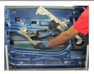
**STEP 3:** Install the right side track into the door.
