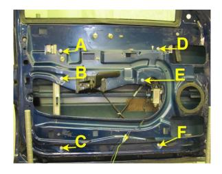
**STEP 9:** Lubricate the window run channels.
