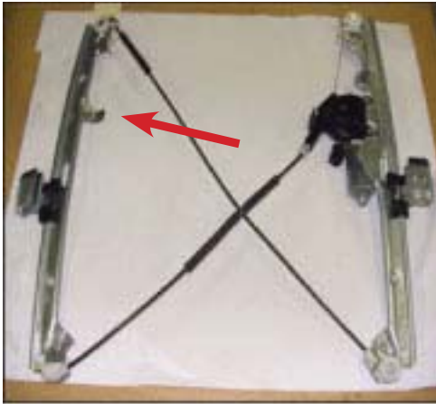
Original Equipment Has 3rd Mounting Bracket
