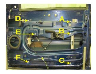
**STEP 9:** Lubricate the window run channels.
