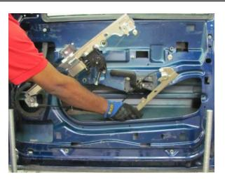
**STEP 3:** Install the left side track into the door.
