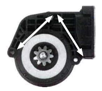
Many OEM & replacement regulators have an elongated third hole that will accept motors with either the 62mm or the 66mm measurement.
