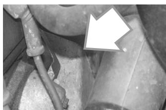
If equipped, remove firewall-mounted heat shield.
