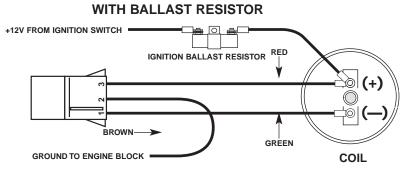
NOTE— If your vehicle is difficult to start, remove the red wire from the plus (+) side of the ignition coil and connect it to the ignition switch side of the ballast resistor..
