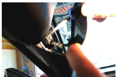
3. There is a safety strap that needs to be removed to pull the pillar away. The screwdriver is pressing into the point where it is released in this picture.
