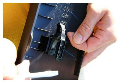
The safety strap is then removed from the factory pillar. The tab on the back is depressed and it slides right out.
